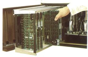
System Three computer is constructed so that hinged front panel swings open and mother-board/card cage slide out for easy insertion of circuit boards.
