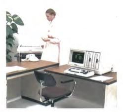
All components of the EW-100 are designed for table top operation. The electronic keyboard is separate from the CRT and allows the operator to adjust its position for maximum personal comfort. This component design feature provides for optimum location compatibility and operational convenience.
