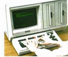
The EW-100 has conveniently incorporated a glossary function which enables the operator to quickly call up prestored words, sentences or paragraphs for insertion into the text. A total of up to 52 different glossaries can be called out by simply depressing the CTRL key and an upper case or lower case letter of the alphabet at the same time. This feature is especially convenient when preparing documents with standardized elements of text such as contracts.
