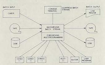
Concurrently, multiple programs are being executed in the foreground. Two terminals are working with COGO-11, one with STRESS-11, one with PLOT-11, one with EDITOR, and one terminal is running a previously-compiled, user written program. The user working with the EDITOR may be preparing programs for later execution in FORTRAN, MACRO, or any other language. Or he could be interactively creating data files for use in another program.
