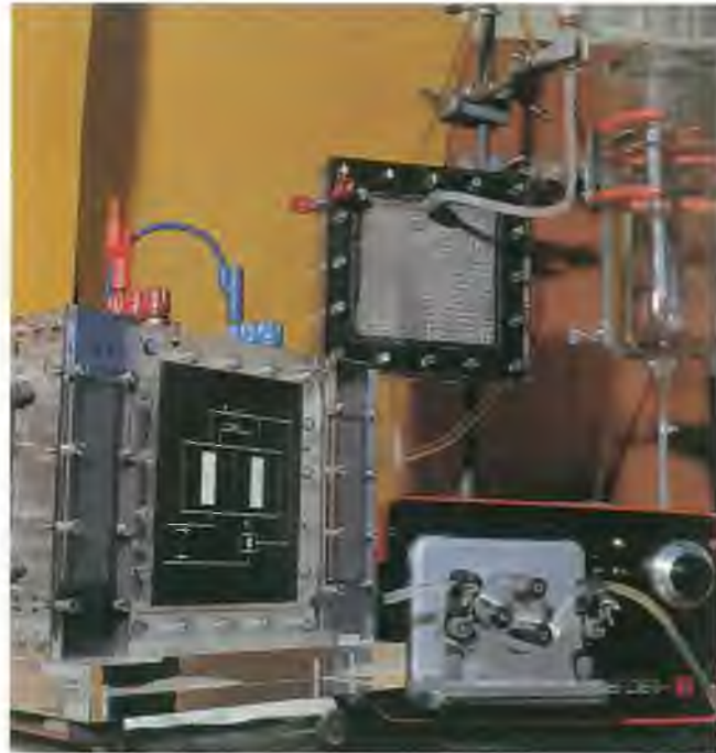
Test rig of a laboratory cell for the electrochemical elimination of urea.
