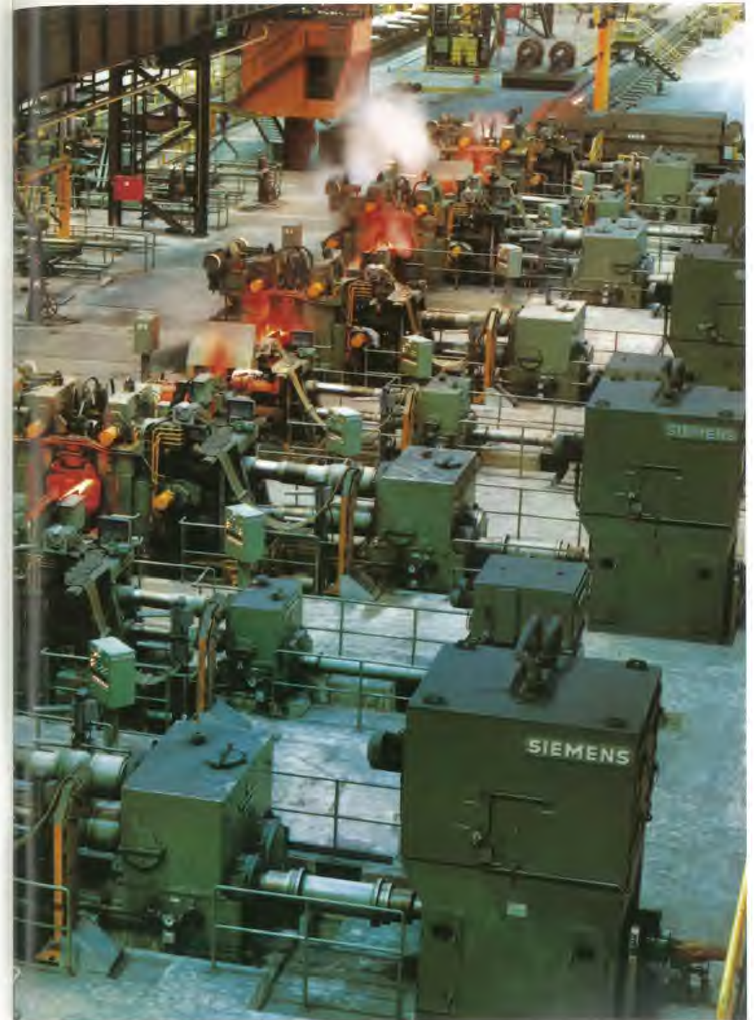
Computer-controlled high-capacity universal mill for the manufacture of girders in the steelworks of Peine-Salzgitter AG. Our picture shows the control pulpit, mill motors, and shear drive. ▷
