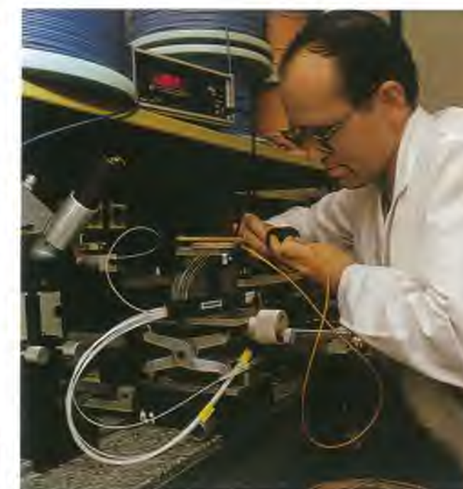
Measurement of light distribution at a coupling network for the optical transmission of information.
