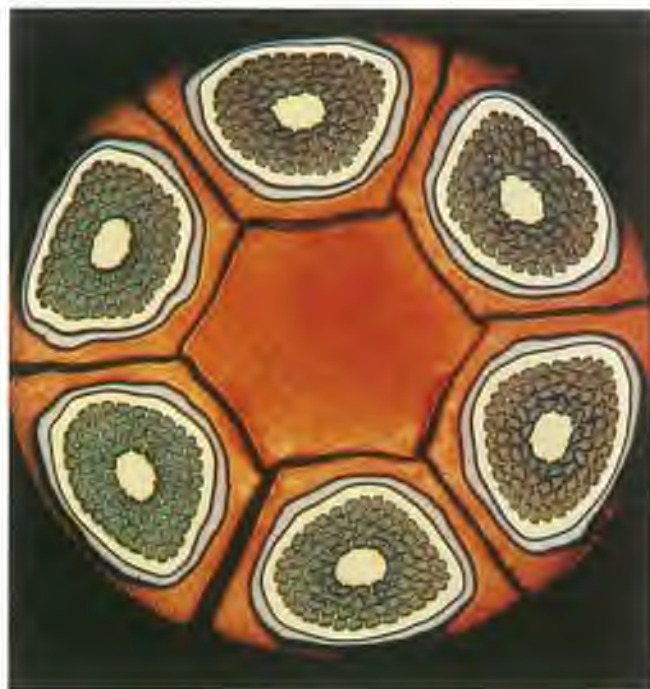
Six-element wire with niobium-tin conductors arranged around a copper core (manufactured by VAC)
