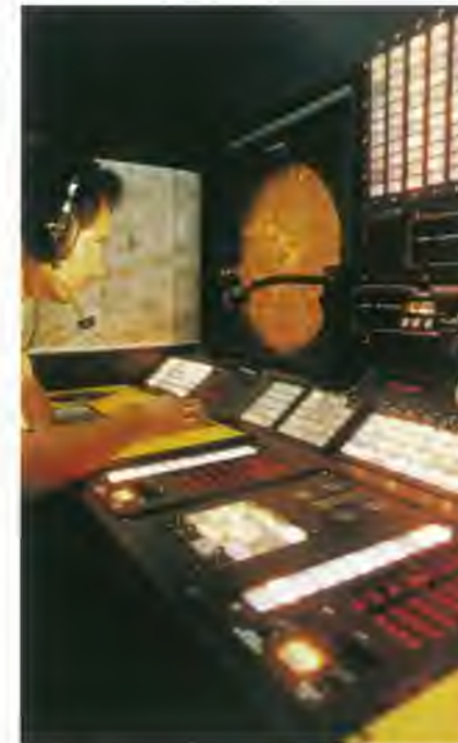
Reliable air space surveillance: Aircraft movements over widespread areas are displayed in this control room.
