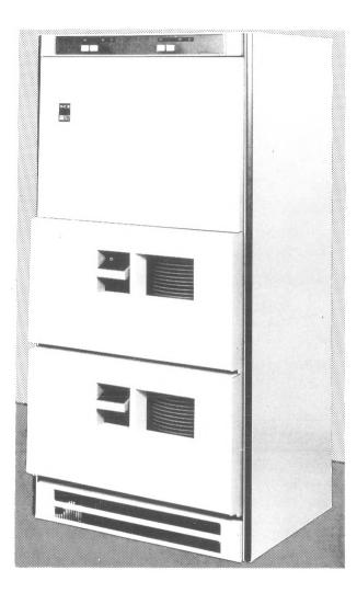
The 657 Disc Unit is available in either a single or dual spindle model, each spindle holding a removable, 20-surface disc pack. Up to four disc units (eight spindles) can be interfaced to a single trunk position through the 625-201 Control Unit, which records data at a density of 2200 bpi and has a maximum transfer rate of 315 kb.
