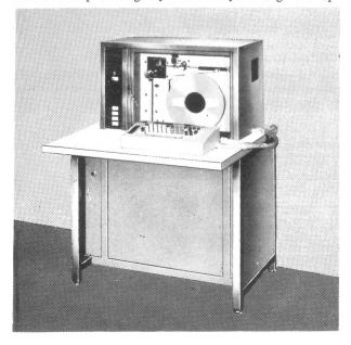
Magnetic tape encoders offer a convenient way to increase system throughput by encoding and verifying directly from source documents to magnetic tape on the same unit. Verified output from these encoders is immediately available for input to NCR Century systems. Other models can perform such functions as prooftape printing, report printing, control total accumulation, punched tape or card to magnetic tape conversion, or remote data transmission offline.
