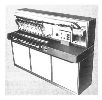
per minute into 11 pockets. The 671 reader/sorter can sort up to 1200 documents per minute into 17 pockets. Both peripherals operate in either an online or offline environment.
