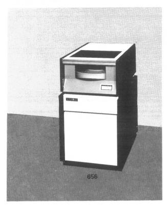
The 656 Disc Unit is a single spindle unit that holds one removable, and optionally one fixed, 2 surface disc cartridge. Each disc cartridge has a capacity of almost 5 million bytes. The disc drive, common trunk control unit and power supply are all housed in one low profile cabinet. If the fixed cartridge option is taken, almost 10 million bytes of directly accessible storage are provided per disc unit.
